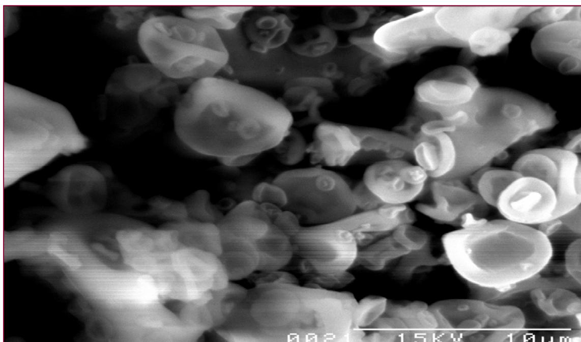
**Scanning electron micrograph of spray dried microcapsules**
